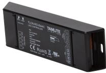
To supply Tamlite's TLCN Series of RF Controls as specified. The 4 channel 5A Constant Voltage RF Receiver shall operate at 12-36Vdc. To be used to control low voltage luminaires when paired with an appropriate Tamlite RF controller. Communication Frequency - 916.66 MHz (Transmission distance 30 Meters Max). The RF Receiver shall be cRU listed.
