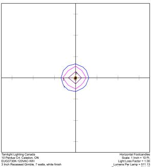
Horizontal Footcandles Scale: 1 Inch = 10 Ft. Light Loss Facie: 1 Ft. Lumens Per Lamp = 511.13 Total Lamp Lumens = 511.13 Mounting Height = 10.00 Ft. Maximum Calculated Value = 12.30 Fc. Arrangement: Single
