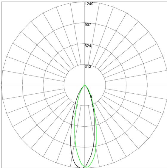
Maximum Candela = 1248.77 Located At Horizontal Angle = 180, Vertical Angle = 2
