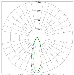
Maximum Candela = 1248.77 Located At Horizontal Angle = 180, Vertical Angle = 2 # 1 - Vertical Plane Through Horizontal Angles (0 - 180) # 2 - Vertical Plane Through Horizontal Angles (90 - 270)
