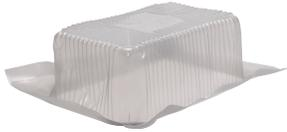
To supply Tam-lite DLVBL series of Large Vapour Barriers as specified. The vapour barrier is for use with Tam-lite DL5, DL6 series recessed pot lights as well as ceiling mounted Speakers and Fans to prevent air leakage from your living space into the attic. Suitable for insulated ceilings. For use in new construction applications.
