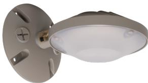
To supply Tamlite TLDD Series of outdoor LED Dusk to Dawn Fixture as specified. The luminaire shall operate at 120Vac and use a NICHIA® Approved Driver. The housing shall be constructed of powder coated die-cast aluminum with a gasketed polycarbonate lens. A durable formed gasket shall be provided between the enclosure and the lens. All parts shall be corrosion resistant. The LEDs shall be supplied with the luminaire. The fixture shall be c-ULus approved and DLC Listed.
