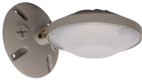
To supply TamLite TLDD Series of outdoor LED Dusk to Dawn Fixture as specified. The luminaire shall operate at 120Vac and use a NICHIA® Approved Driver. The housing shall be constructed of powder coated die-cast aluminum with a gasketed polycarbonate lens. A durable formed gasket shall be provided between the enclosure and the lens. All parts shall be corrosion resistant. The LEDs shall be supplied with the luminaire. The fixture shall be c-ULus approved and DLC Listed.
