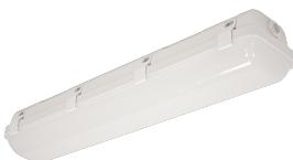
To supply Tamlite VPS Contractor Series of LED vapour proof fixtures as specified. The luminaire shall operate at 120-347Vac. The housing shall be constructed of Bayer® polycarbonate with a clamp down opal Bayer® polycarbonate lens. The fixture shall be IP65 rated and include an IP66 strain relief. A durable formed gasket shall be provided between the enclosure and the lens. All parts shall be corrosion resistant. The LED shall be supplied with the luminaire. The fixture shall be cULus Listed.
