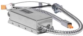
To supply Tamlite's TLD Series of LED Commercial Retrofit Whip as specified. The housing shall operate at 347Vac as specified and use a 1-10V dimmable, constant current type driver. Cable connections between light engine and driver shall use armoured cable. Retrofit Whip shall be c-ULus listed.
