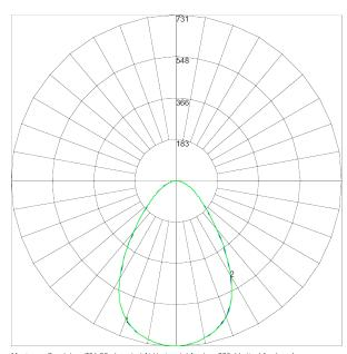
Maximum Candela = 731.28 Located At Horizontal Angle = 225, Vertical Angle = 1 # 1 - Vertical Plane Through Horizontal Angles (225 - 45) (Through Max. Cd.) # 2 - Vertical Plane Through Horizontal Angles (0 - 180)
