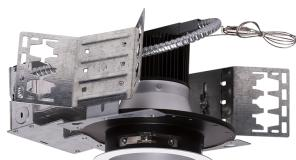
To supply Tamlite's TLD Series of LED Architectural Commercial Housing with Trims as specified. The housing shall operate at 347Vac and use a 1-10V dimmable, constant current type driver. Cable connections between light engine and driver shall use armored cable. Reflector shall be constructed of spun and die cast Aluminium. The LEDs shall be 1-10V Dimmable. Housing and Trim shall be c-UL-us listed.
