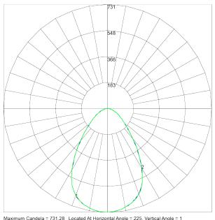
Maximum Candela = 731.28 Located At Horizontal Angle = 225, Vertical Angle = 1 # 1 - Vertical Plane Through Horizontal Angles (225 - 45) (Through Max. Cd.) # 2 - Vertical Plane Through Horizontal Angles (0 - 180)
