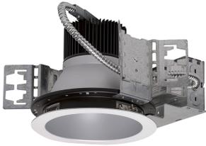
To supply Tamlite's TLD Series of LED Architectural Commercial Housing with Trims as specified. The housing shall operate at 347Vac and use a 1-10V dimmable, constant current type driver. Cable connections between light engine and driver shall use armored cable. Reflector shall be constructed of spun and die cast Aluminium. LEDs shall be as specified EVERLIGHT® 62-217B LED chips. The LEDs shall be 1-10V Dimmable. Housing and Trim shall be c-UL-us listed.
