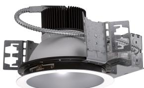
To supply Tamlite's TLD Series of LED Architectural Commercial Housing with Trims as specified. The housing shall operate at 347Vac and use a 1-10V dimmable, constant current type driver. Cable connections between light engine and driver shall use armored cable. Reflector shall be constructed of spun and die cast Aluminium. LEDs shall be as specified EVERLIGHT® 62-217B LED chips. The LEDs shall be 1-10V Dimmable. Retrofit Whip and Trim shall be c-UL-us listed.
