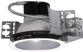
To supply Tamlite's TLD Series of LED Architectural Commercial Housing with Trims as specified. The housing shall operate at 347Vac and use a 1-10V dimmable, constant current type driver. Cable connections between light engine and driver shall use armored cable. Reflector shall be constructed of spun and die cast Aluminium. LEDs shall be as specified EVERLIGHT® 62-217B LED chips. The LEDs shall be 1-10V Dimmable. Retrofit Whip and Trim shall be c-UL-us listed.
