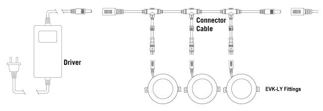
$The \ Kit is sold as shown with three (3) \ EVK-LY \ fittings. The power supply can be loaded to a max of four (4) \ EVK-LY \ fittings.$
