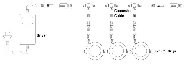
$The \ Kit is sold as shown with three (3) \ EVK-LY fittings. The power supply can be loaded to a max of four (4) \ EVK-LY fittings.$
