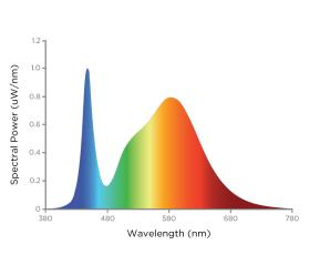
Source Type: LED CRI: >80 Chromaticity: x=0.3803 y=0.3817 Manufacturer: Everlight® L90: 54,000 Hrs Colour Tolerance: 3 SDCM Part Number: 67-21S Colour Temperature: 4000K Duv: 0.0023
