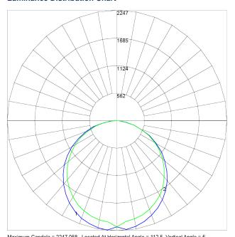
Maximum Candela = 2247.058 Located At Horizontal Angle = 112.5, Vertical Angle = 5 # 1 - Vertical Plane Through Horizontal Angles (112.5 - 292.5) (Through Max. Cd.) # 2 - Vertical Plane Through Horizontal Angles (0 - 180)
