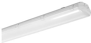
To supply TamLite TLVP Series of LED vapour proof fixtures as specified. The luminaire shall operate at 347Vac. The housing shall be constructed of Bayer® polycarbonate with a clamp down opal Bayer® polycarbonate lens. The fixture shall be IP65 rated and include an IP66 strain relief. A durable formed gasket shall be provided between the enclosure and the lens. All parts shall be corrosion resistant. The LED shall be supplied with the luminaire. The fixture shall be cULus & DLC Listed.
