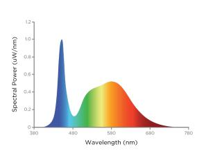
Source Type: LED Colour Temperature: 3000K, 4000K, 5000K Field Selectable
