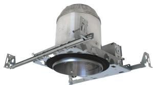
To supply and install Tamlite DL5MED Series of line voltage recessed Housing as specified. The Housing shall operate at 120Vac. Lamps shall be as specified, medium base lamps up to a maximum of the rated lamp wattage on the fixture nameplate. The lamps shall not be supplied with the fixture. The fixture shall be c-UL-us approved.
