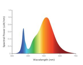
Source Type: LED CRI: >70 Chromaticity: x=0.4370 y=0.4041 Manufacturer: Nichia® L70: 60000 Hrs. Colour Tolerance: 3 SDCM Part Number: NVSW219 Colour Temperature: 3000K Duv: 0.0018
