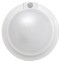
To supply Tamlite RFJ Series of LED Recessed downlights as specified. The fixture shall operate at 120Vac. LED'S shall be as specified, SEOUL® STWxC2SB LED Chips with a CRI of over 90 for increased colour rendering. Housing shall be constructed of die cast aluminum. The fixture shall be suitable for damp locations and controlled by Passive infra red sensors at 120Vac. The fixture shall be cETLus approved and Energy Star Listed.
