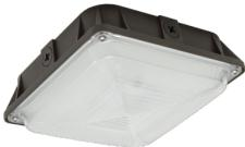
To supply Tamlite's TLC Series of LED Canopy fixture as specified. The luminaire shall operate at 120-277Vac. The housing shall be constructed of Die-Cast Aluminium with a powder coat finish over chromate conversion treatment with a clear polycarbonate lens. The luminaire shall be wet location listed. LEDs shall be as specified NICHIA® LED chips. The luminaire shall be cULus Listed.
