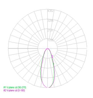
Initial Lumen Output: 2723lm Beam Angle: 38 deg UL Classification: Wet Location Listed DLC Number: DDDIPB Efficacy: 106.0lm/W Field Angle: 83 deg Ambient Operating Temp: -40C to +40C CCN Number: IFAM7.E359675 CBCP: 4379cd Environmental Rating(s): IP65 Certification Standards: UL Safety US-CA , DLC Limited Product Warranty: 5 Year(s)
