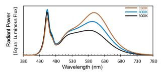
Source Type: LED **L90:** > 50,000 hrs. Colour Temperature: 3000K, 3500K, 4000K, 5000K Field Selectable
