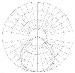
Maximum Candela = 562.19 Located At Horizontal Angle = 180, Vertical Angle = 18 # 1 - Vertical Plane Through Horizontal Angles (0 - 180) # 2 - Vertical Plane Through Horizontal Angles (90 - 270)
