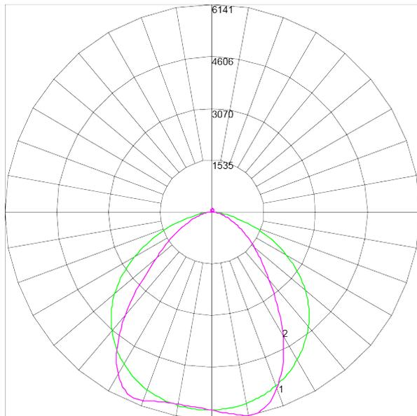
Maximum Candela = 6140.73 Located At Horizontal Angle = 360, Vertical Angle = 11
