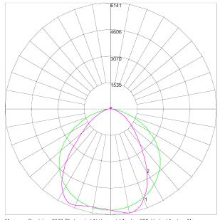
Maximum Candela = 6140.73 Located At Horizontal Angle = 360, Vertical Angle = 11 # 1 - Vertical Plane Through Horizontal Angles (90 - 270) # 2 - Vertical Plane Through Horizontal Angles (0 - 180)
