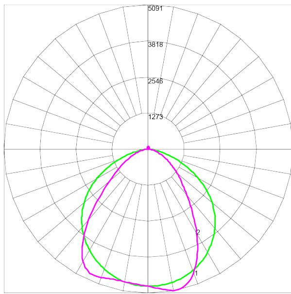
Maximum Candela = 5091.216 Located At Horizontal Angle = 0, Vertical Angle = 11
