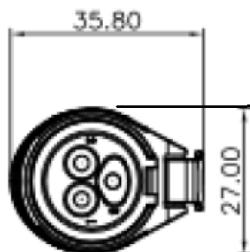
5-Pole IP65 Metal Connector Female. Cable size; 8-12mm (0.3149 - 0.4724 inches) , 12A 500V rated
