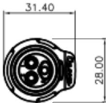
5-Pole IP65 Metal Connector Male Cable size; 8-12mm (0.3149 - 0.4724 inches) , 12A 500V rated
