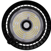
To supply the Tamlite HBM Series selectable white LED high bay luminaire as specified. The luminaire shall operate at 120-347Vac. The fixture is 0-10Vdc dimmable with optional sensor. Wattage is field selectable to three levels. CCT is field selectable to three levels. The housing shall be constructed of aluminum with a prismatic lense. LEDs shall be as specified Lumileds® LED chips. The luminaire shall be cULus Listed.
