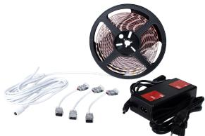
To supply Tamlite EVKTP series of single colour LED Tape light. Tape shall use an integrated SMD LED cluster. Tape shall be cuttable in intervals of 4 inches (101.6mm) and be sold in lengths of 5M. Plug-in driver shall be external. Kit shall come with driver, wiring and connectors. Tape Light Kit shall be cETLus approved.
