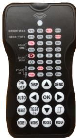
The Tamlite Z10 Remote Control is used to program the Z10 Senso from the ground. It allows for preset modes as well as customization of various settings. Occupancy, Day Light, Sensitivity, Timeframe.
