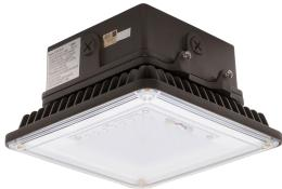
To supply Tamlite's DLC Series of LED Canopy fixture as specified. The luminaire shall operate at 347Vac. The housing shall be constructed of Die-Cast Aluminium with a powder coat finish over chromate conversion treatment with a clear polycarbonate lens. The luminaire shall be wet location listed. LEDs shall be as specified NICHIA® LED chips. The luminaire shall be cULus Listed.
