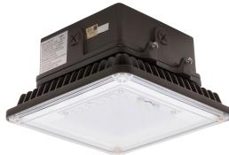
To supply Tamlite's TLC Series of LED Canopy fixture as specified. The luminaire shall operate at 347Vac. The housing shall be constructed of Die-Cast Aluminium with a powder coat finish over chromate conversion treatment with a clear polycarbonate lens. The luminaire shall be wet location listed. LEDs shall be as specified NICHIA® LED chips. The luminaire shall be cULus Listed.
