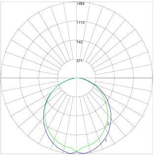
Maximum Candela = 1484.22 Located At Horizontal Angle = 90, Vertical Angle = 5 # 1 - Vertical Plane Through Horizontal Angles (90 - 270) (Through Max. Cd.) # 2 - Vertical Plane Through Horizontal Angles (0 - 180)
