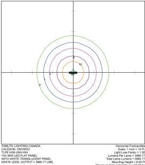
Honizontal Footcandles Scale: 1 Inch = 10 Ft. Light Loss Factor = 1.00 Lumens Per Lamp = 3880.77 Total Lamp Lumens = 3880.77 Mounting Height = 8.00 Ft Maximum Calculated Value = 22.52 Fc Arrangement: Single
