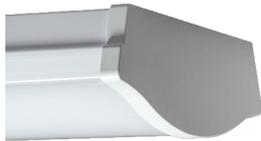
To supply Tamlite TLCR series of LED Wrap fixtures as specified. The luminaire shall operate at 347Vac. The housing shall be constructed of powder-coated aluminum with a heat and impact resistant tempered PMMA lens. All parts shall be corrosion resistant. The LEDs shall be supplied with the luminaire. The fixture shall be c-ULus listed.
