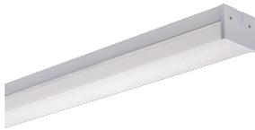
To supply TamLite TLWR series of LED Wide Wrap fixtures as specified. The luminaire shall operate at 120-277Vac. The housing shall be constructed of powder-coated Aluminium with a heat and impact resistant tempered PMMA lens. All parts shall be corrosion resistant. The LEDs shall be supplied with the luminaire. The fixture shall be cULus Listed.
