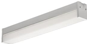
To supply Tamlite TLNR series of LED Wrap fixtures as specified. The luminaire shall operate at 347Vac. The housing shall be constructed of powder-coated Aluminium with a heat and impact resistant tempered PMMA lens. All parts shall be corrosion resistant. The LEDs shall be supplied with the luminaire. The fixture shall be cULus Listed.
