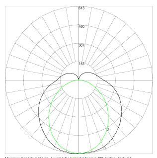
Maximum Candela = 613.28 Located At Horizontal Angle = 180, Vertical Angle = 5 # 1 - Vertical Plane Through Horizontal Angles (0 - 180) # 2 - Vertical Plane Through Horizontal Angles (90 - 270)
