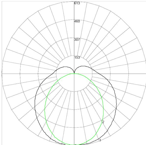
Maximum Candela = 613.28 Located At Horizontal Angle = 180, Vertical Angle = 5
