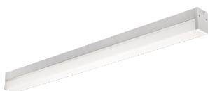
To supply Tamlite TLNR series of LED Wrap fixtures as specified. The luminaire shall operate at 120-277Vac. The housing shall be constructed of powder-coated Aluminium with a heat and impact resistant tempered PMMA lens. All parts shall be corrosion resistant. The LEDs shall be supplied with the luminaire. The fixture shall be cULus Listed.
