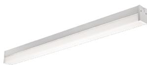
To supply Tamlite TLNR series of LED Wrap fixtures as specified. The luminaire shall operate at 120-347Vac. The housing shall be constructed of powder-coated Aluminium with a heat and impact resistant tempered PMMA lens. All parts shall be corrosion resistant. The LEDs shall be supplied with the luminaire. The fixture will be complete with an integral microwave occupancy sensor and be programable by remote control. The fixture shall be cULus Listed.
