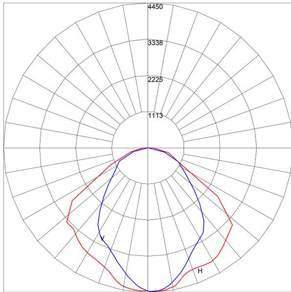
Maximum Candela = 4450.26 Located At Horizontal Angle = 1, Vertical Angle = 3
