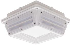
To supply Tamlite's TLG Series of LED Garage fixture as specified. The luminaire shall operate at 120-347Vac. The housing shall be constructed of Die-Cast Aluminium with a powder coat finish over chromate conversion treatment with clear, acrylic lenses. The luminaire shall be wet location listed. LEDs shall be as specified Nichia ® LED chips. The luminaire shall come prewired with a Z-10 Socket. The luminaire shall be cULus Listed.
