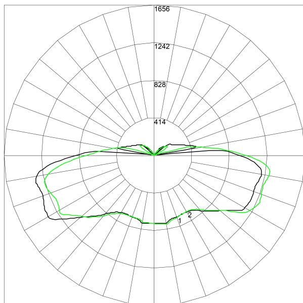
Maximum Candela = 1655.9 Located At Horizontal Angle = 135, Vertical Angle = 69
