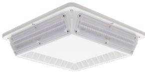
To supply Tamlite's TLG Series of LED Garage fixture as specified. The luminaire shall operate at 347Vac. The housing shall be constructed of Die-Cast Aluminium with a powder coat finish over chromate conversion treatment with clear, acrylic lenses. The luminaire shall be wet location listed. LEDs shall be as specified Nichia ® LED chips. The luminaire shall be cULus Listed and DLC Listed.
