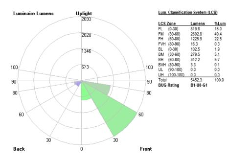
Initial Lumen Output: 5452lm Luminaire Type: Type II-H - Medium UL Classification: Wet Location Listed
