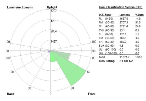
Initial Lumen Output: 11070lm Luminaire Type: Type II-H - Medium **UL Classification:** Wet Location Listed
