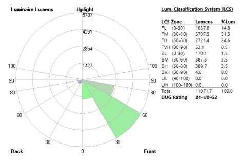
Initial Lumen Output: 11070lm Luminaire Type: Type II-H - Medium UL Classification: Wet Location Listed CCN Number: IFAM7.E359675 Efficacy: 81lm/W BUG Rating: B1-U0-G2 Ambient Operating Temp: -40C to +40C Limited Product Warranty: 10 Year(s) Max Candela: 9385cd (80 h, 71.5V) Environmental Rating(s): IP66 Certification Standards: UL Safety US-CA
