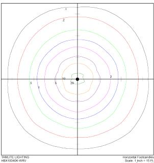
Horizontal Footcandles Scale: 1 Inch = 15 Ft. Light Loss Factor = 1.00 Lumens Per Lamp = N.A. (absolute photometry) Luminaire Lumens = 1435 Mounting Height = 15.00 Ft. Maximum Calculated Value = 23.93 Fc Arrangement: Single
