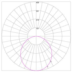
Maximum Candela = 428.5 Located At Horizontal Angle = 0, Vertical Angle = 0 # 1 - Vertical Plane Through Horizontal Angles (0 - 180) (Through Max. Cd.) # 2 - Vertical Plane Through Horizontal Angles (90 - 270)
