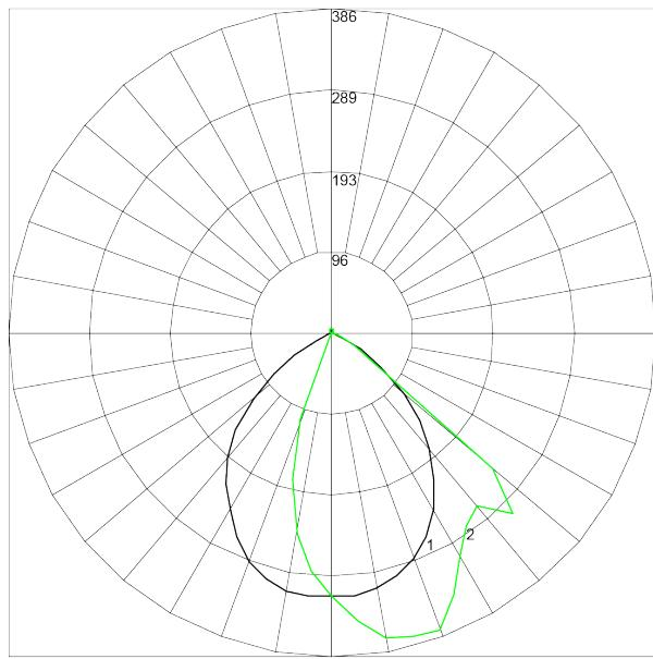
Maximum Candela = 385.54 Located At Horizontal Angle = 112.5, Vertical Angle = 20
