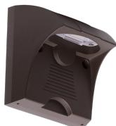
To supply Tamlite's SLSQ Series of LED Square Step Light Luminaire as specified. The luminaire shall operate at 120-277Vac. The housing shall be constructed of powder coated diecast Aluminium with impact resistant polycarbonate lens. The LEDs shall be as specified LUMILEDS® LUXEON 3030 2D LED chips. The luminaire shall be cULus Listed.
