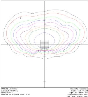
Horizontal Footcandles Scale: 1 Inch = 1.5 Ft Light Loss Factor = 1.00 Lumens Per Lamp = 559.1 Total Lamp Lumens = 559.1 Mounting Height = 1.50 Ft Maximum Calculated Value = 151.77 Fc Arrangement: Single
