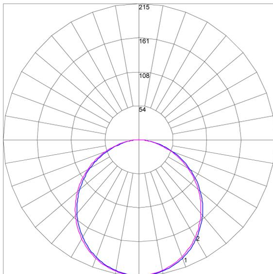
Maximum Candela = 215.002 Located At Horizontal Angle = 315, Vertical Angle = 1
