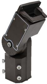
To supply Tamlite's FLX Series 2-3/8" slip-fitter adapter for the FLX series flood lights. The fitting shall be constructed of powder-coated die-cast Aluminium with stainless steel hardware. Universal fit to all wattages of FLX series floodlights.
