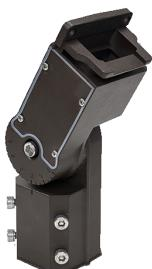
To supply Tamlite's FLX Series 2-3/8" slip-fitter adapter for the FLX series flood lights. The fitting shall be constructed of powder-coated die-cast Aluminium with stainless steel hardware. Universal fit to all wattages of FLX series floodlights.
