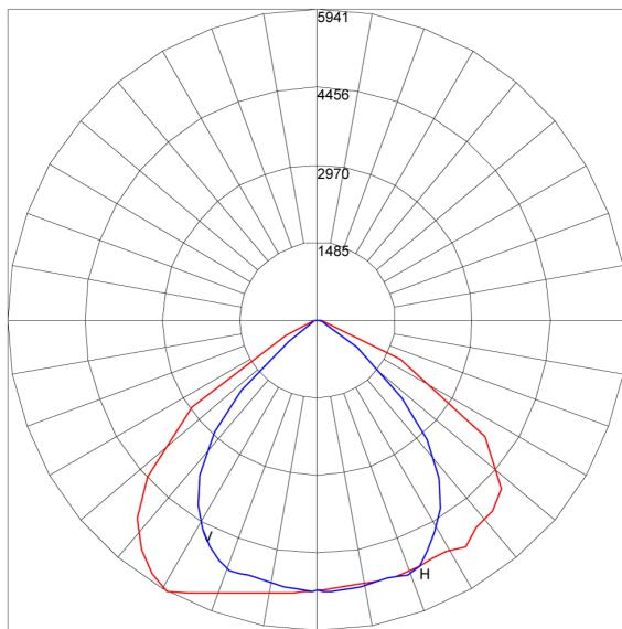
Maximum Candela = 5940.872 Located At Horizontal Angle =-29, Vertical Angle = 0
