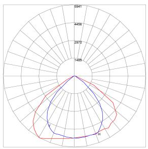
Maximum Candela = 5940.872 Located At Horizontal Angle =-29, Vertical Angle = 0 H - Horizontal Axial Candela V - Vertical Axial Candela
