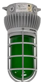
To supply Tamlite CVP Series of Protected LED vapour proof fixtures as specified. The luminaire shall operate at 120-277Vac. The housing shall be constructed of die-cast aluminum with a borosilicate glass globe, and die-cast protective cage. The fixture shall be Wet Location listed. A durable formed gasket shall be provided between the enclosure and the globe. All parts shall be corrosion resistant. The fixture shall be c-UL-us approved.
