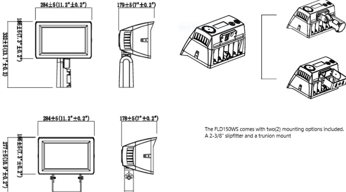
The FLD150WS comes with two(2) mounting options included. A 2-3/8" slipfitter and a trunion mount
